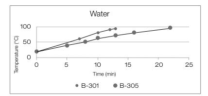
$\Delta T_{_{70\,^{\circ}C\,(water)}}\colon$  B-301 -> 13 min; B-305 -> 22 min
