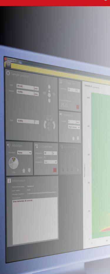
Dedicated software is one of the most important components of a modern SAXS system. SAXSpace comprises three different programs for automated system control and data acquisition as well as fast and easy template-based processing and analysis of 2D and 1D SWAXS data.
